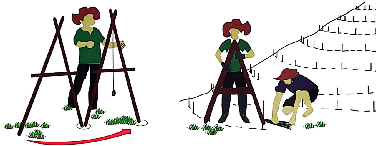
Figure 5b: Laying out a contour line variation
